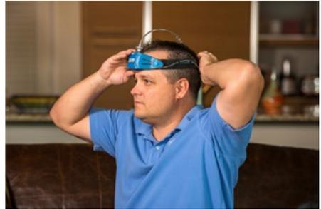
Figure 2. Center the ARES over your nose, slightly above your eyebrows, and gently pull the black strap into place.
